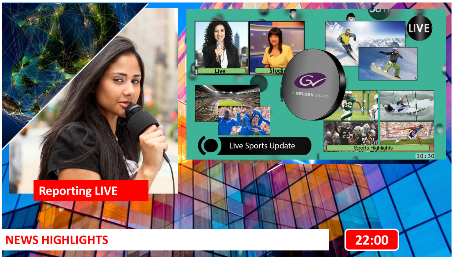
Cascading M/Es — M/E 1 feeding key layer, outputting on M/E 2
